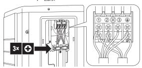
Tighten the terminal screws securely. We recommend using a Phillips screwdriver.
