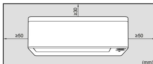
**Note:** Make sure that there are no obstacles within 500 mm under the infrared signal receiver. They may influence reception performance of the wireless remote control.
